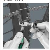
With the included chain tool, chains can be loosened and reconnected; ideal for opening and closing bicycle chains. Suitable for single-speed chains up to 12-speed.
