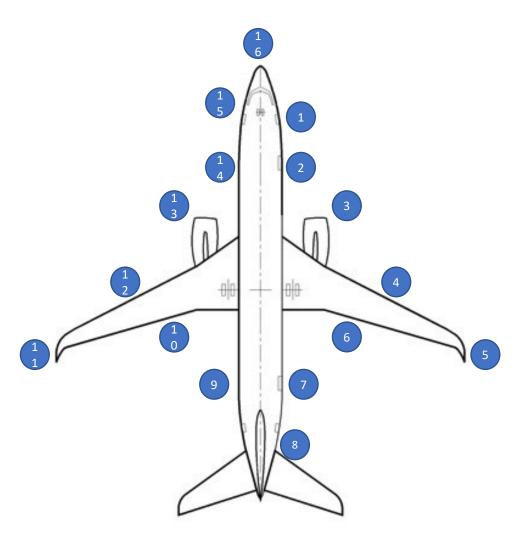
Prior to flight departure, the lead or designee must conduct a walk-around, following the removal of all equipment. You should look specifically at these locations on the aircraft, while being aware of any other noticeable damage or leaks. In the event a piece of equipment or door is re-engaged/opened a re-check of the area is required.
