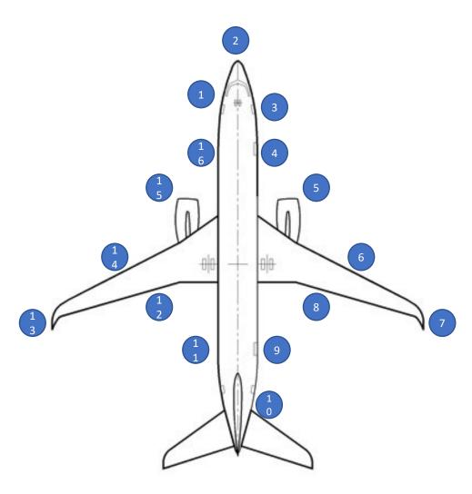
After flight arrival, the lead or designee must conduct a walk-around, prior to any equipment being brought up to the aircraft. You should look specifically at these locations on the aircraft, while being aware of any other noticeable damage or leaks.
