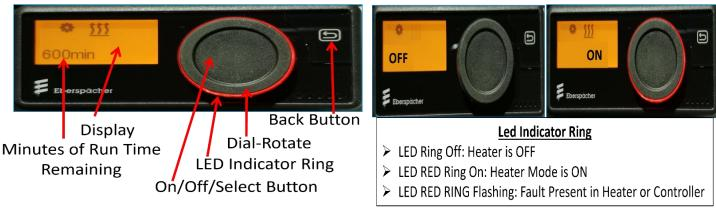
This Bunk Heater is designed to be used in conjunction with the truck's Auto-Start/Opti-Idle management system.
