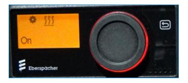
Press the Select button for more than 2 seconds to turn off the controller and the bunk heater.
