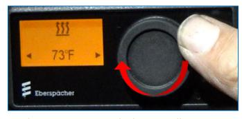
Step 5. Rotate the Dial to adjust the temperature setting.
