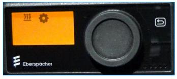
Step 2. If needed rotate the dial to the desired mode setting. Select the **!!!** symbol for the Heating Mode.
