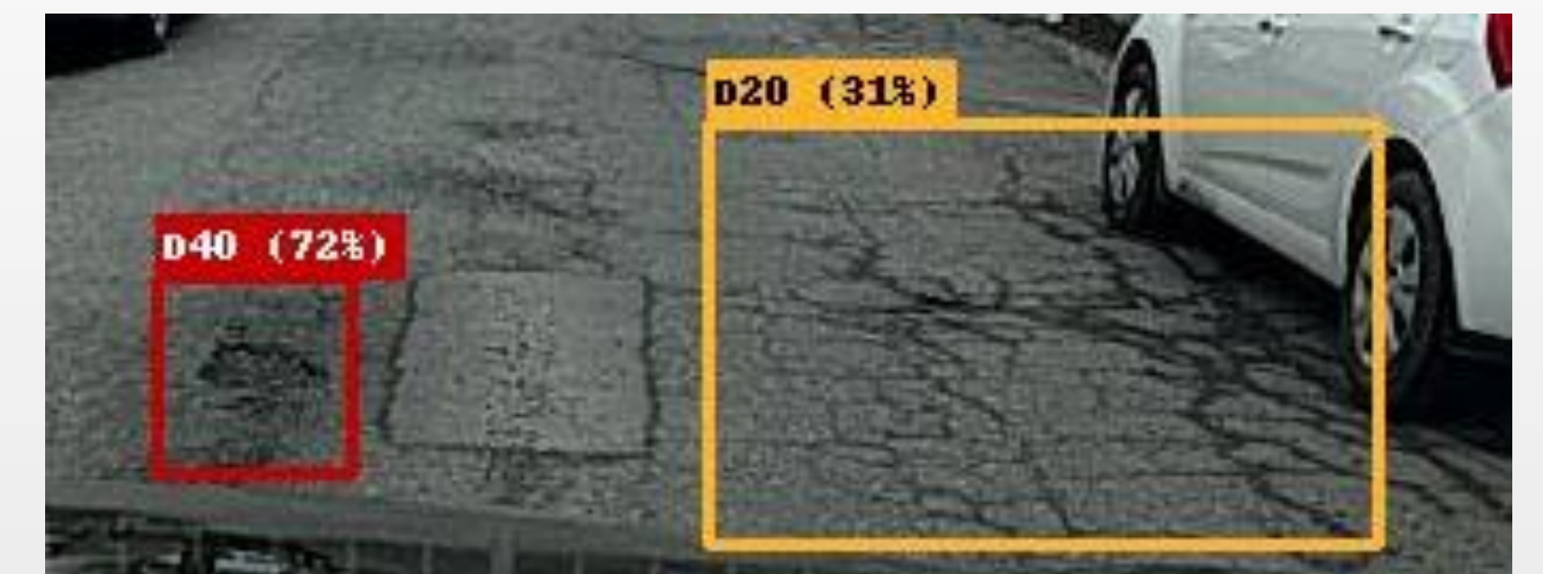
Fig. 3 Prediction of the V01 object detector.
