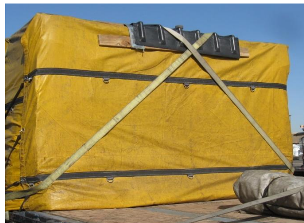
CROSS TIE WITH ASPHALT SHINGELS
