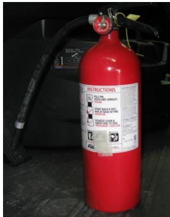
FULLY- CHARGED FIRE EXTINGUISHER
