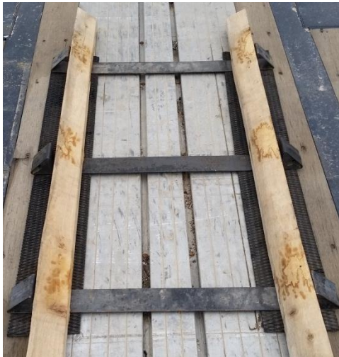
INITIAL COIL RACK SETUP WITH DUNNAGE
