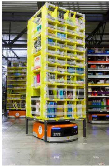
Figure 2.1 Kiva Robot Carrying a Pod to Picker
