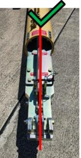
Do not use if the Towing Head is not aligned properly. If the head appears to be at an angle, the shear pins/bolts have failed.
