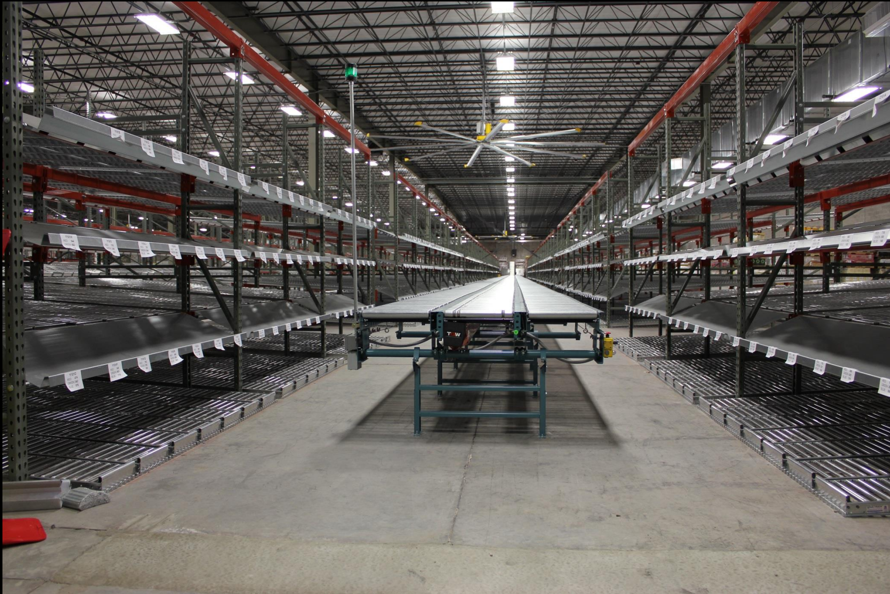
Powered Conveyor with a Carton Flow System
