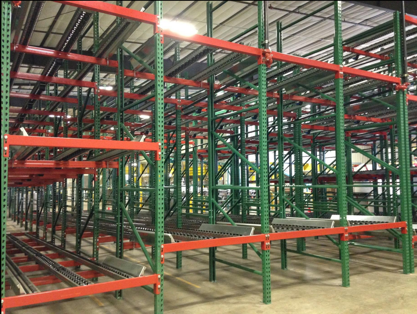
Pallet Flow Pallet Rack - First In - First Out
