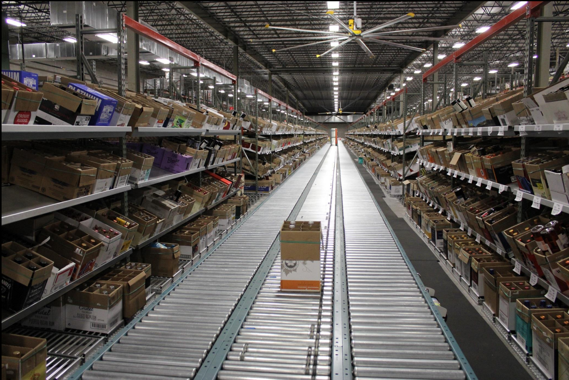
Powered Conveyor with a Carton Flow System
