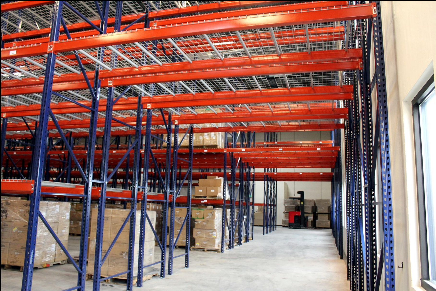
Selective Pallet Rack with Drive-Through Tunnel
